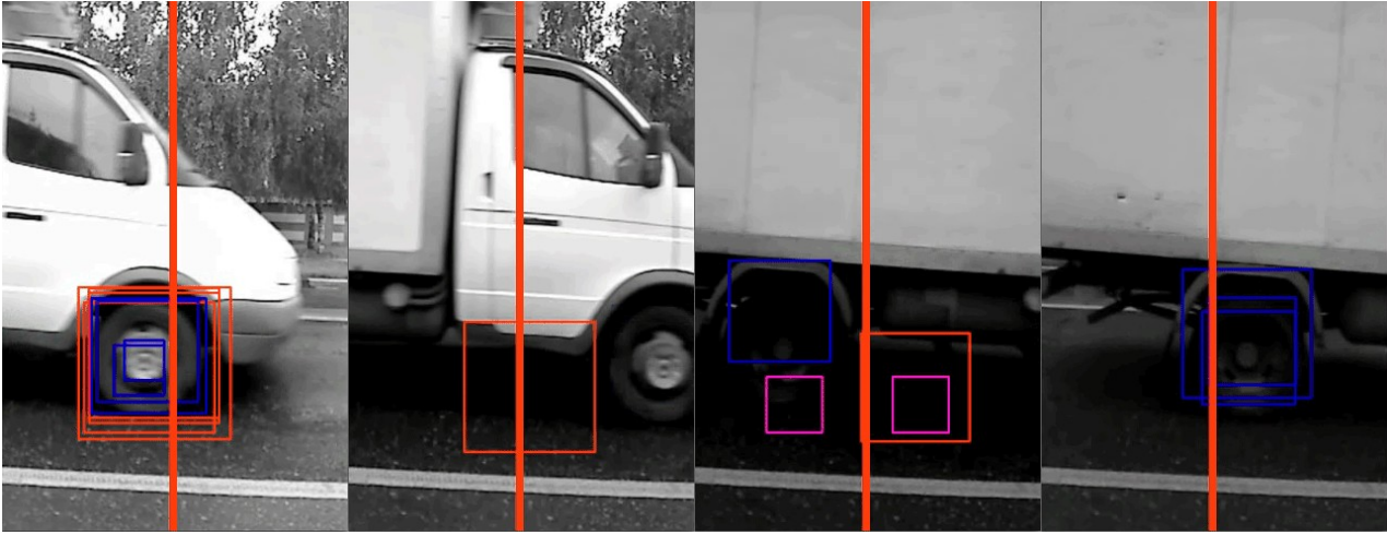
Fig. 1. Vehicle passing near the automatic vehicle classifier camera. Squares show wheel detector results.
