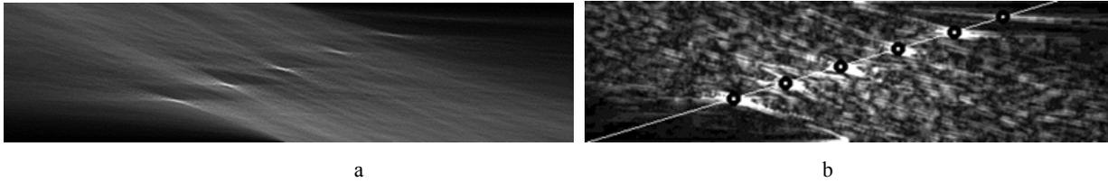
Figure 3. (a) Hough-image; (b) DoG-filtered Hough-image. The straight line corresponds to the vanishing point.
