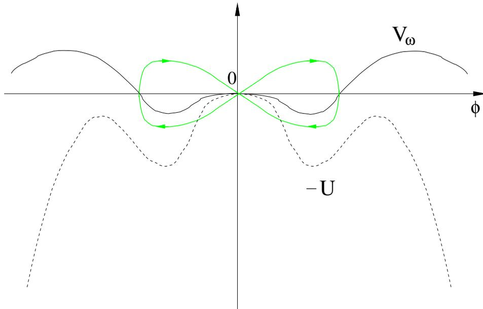
FIGURE 7. Potentials and soliton on the phase plane
