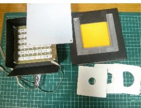
Fig. 2. Stimulus box disassembled
