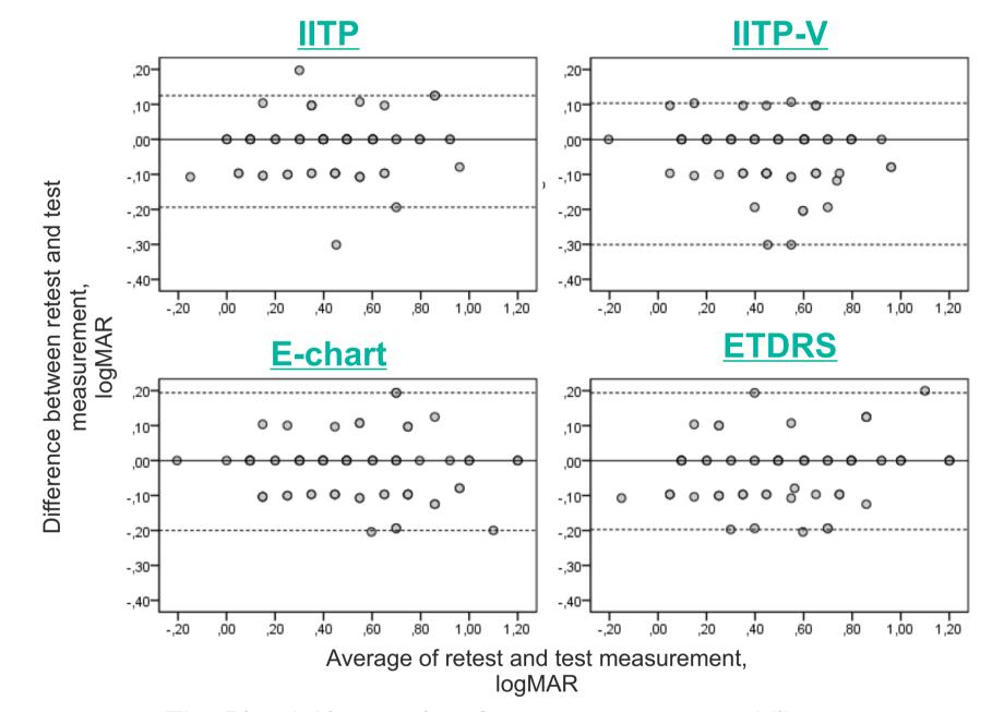
The Bland-Altman plots for test-retest repeatability assessment. The solid line marks the median (zero for all four charts tested). The dashed lines marks 2.5 percentile and 97.5 percentile, so the range between dashed line is 95% limits of agreement (LoA).
